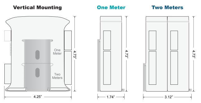
Right Angle Mounting Bracket (part# CHWR-0200) allows for Vertical mounting of 1 or 2 DTS 307 / DTS 310 / DC Meters.
