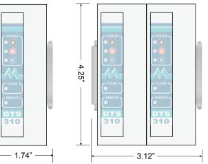
Right Angle Mounting Bracket (part# CHWR-0200) allows for Horizontal mounting of 1 or 2 DTS 307 / DTS 310 / DC Meters.
